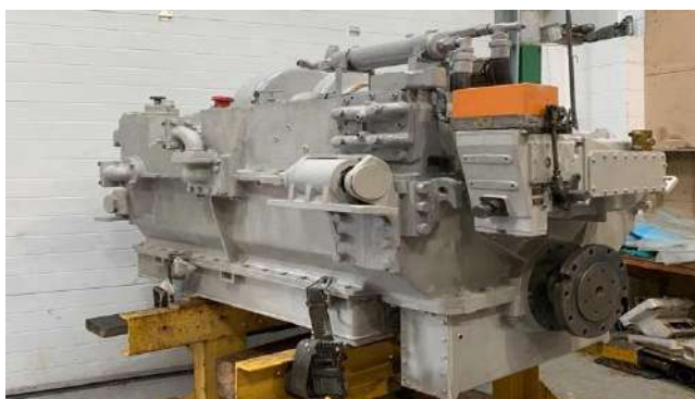
The overhaul of the second of the Voith hydraulic transmissions from D1010 'WESTERN CAMPAIGNER' has now been completed by the DEPG's 'transmission team'. Pictured at Williton on 19 th March 2024 by Andy Royal ©
