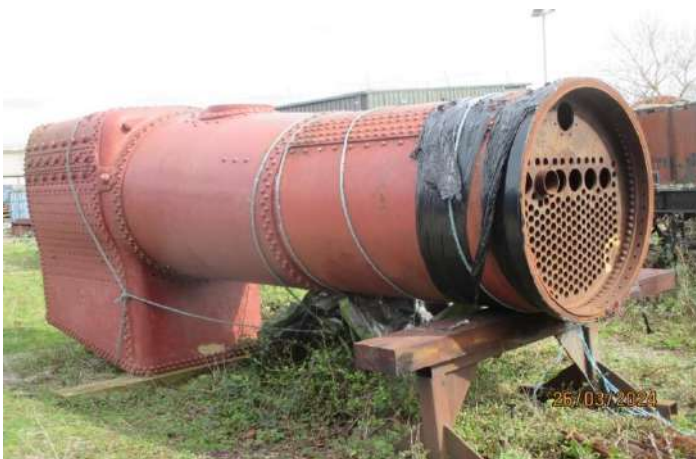
4561 boiler awaiting restoration. [Photo: Geoff Garfield]
