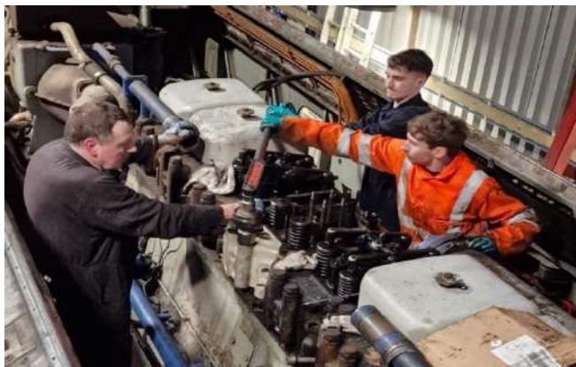
Volunteer loco manager Ian supervises as Ashley and Tom pull on the torque wrench to tighten one of the eight cylinder-head bolts on Class 33 'Crompton' D6575 (33057). Pictured at Williton on 20 th January 2024 by Martin Howard ©
