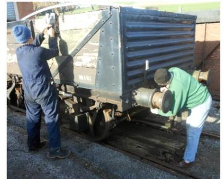
ends and metalwork has been painted olive, which is the correct livery, rather than black. Planks to replace those too rotten to repair
